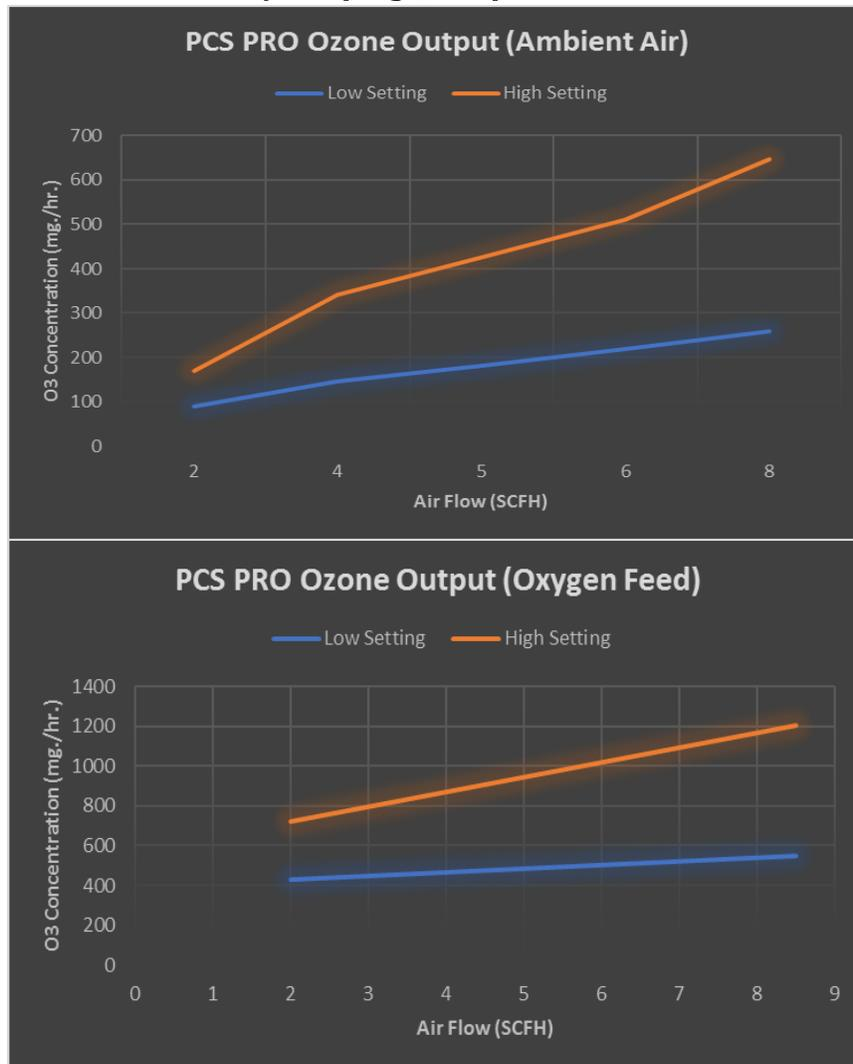
Figure 1: PCS PRO ozone output measured in mg./hr.
