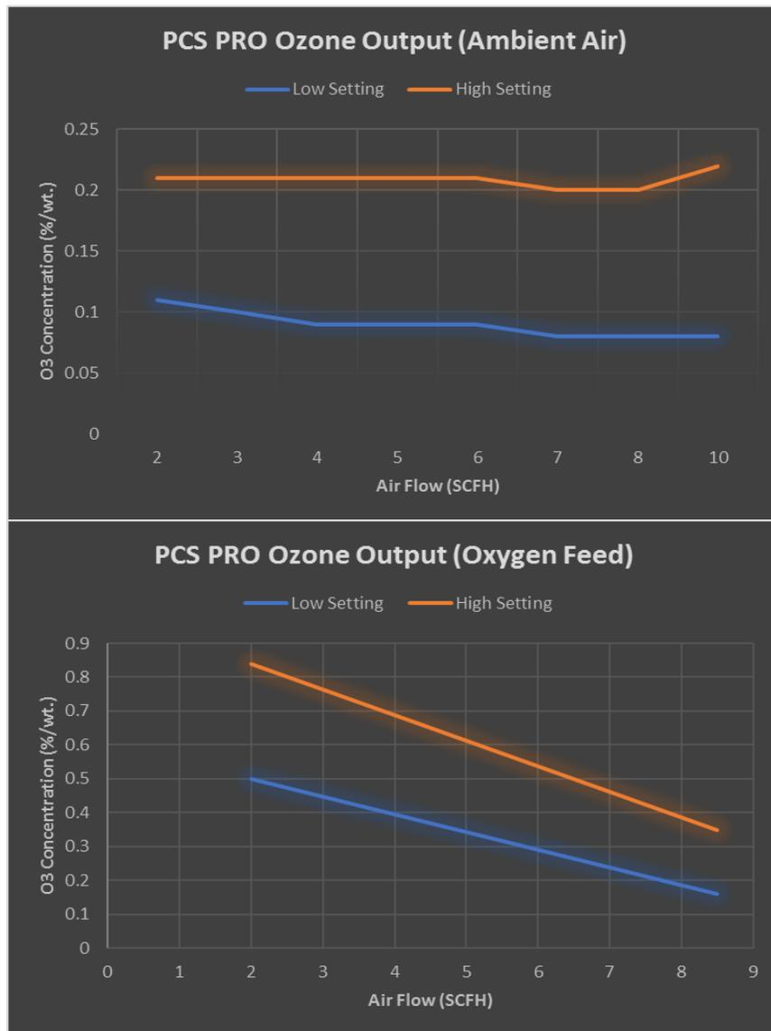
**Figure 2:** PCS PRO ozone output measured in %/wt.
