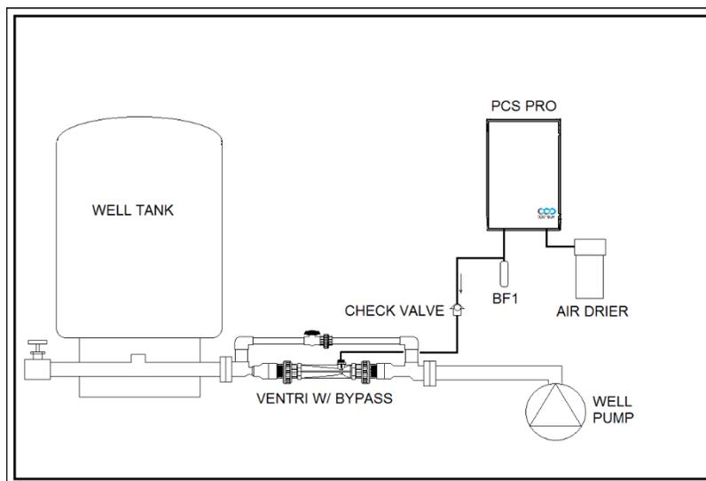
Figure 4: PCS PRO typical use diagram
