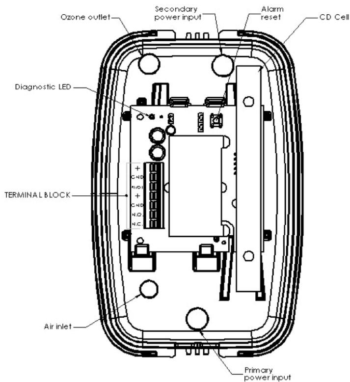
Figure 1: OzotechEOG internal layout
