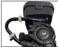
2. Disconnect power to the control valve. Remove the front cover from valve backplate. Release the control board bracket from backplate.
