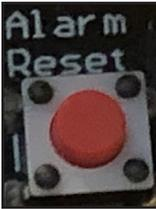
3. Pulsing orange LED will indicate timer rest function is active.\* Press reset button again to complete reset. LED will pulse green when finished.
