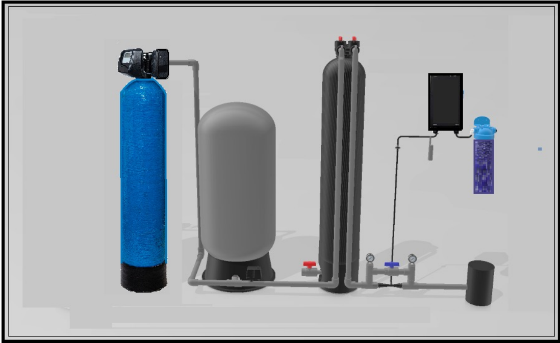
Figure 2. Typical well application w/EOG filter
