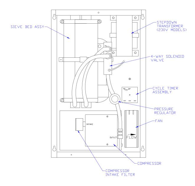
FIGURE 1 - Component Layout Diagram, Power Prep Phoenix, All Models
