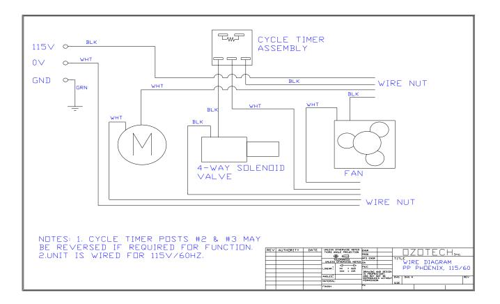
FIGURE 2 - Wiring Diagram, Power Prep Phoenix, 115Vac/60Hz
