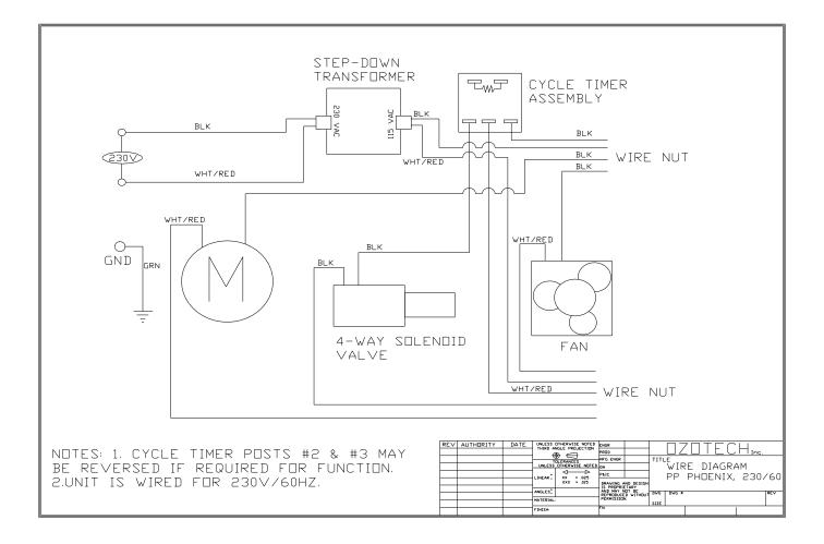
FIGURE 3 - Wiring Diagram, Power Prep Phoenix, 230Vac/60Hz
