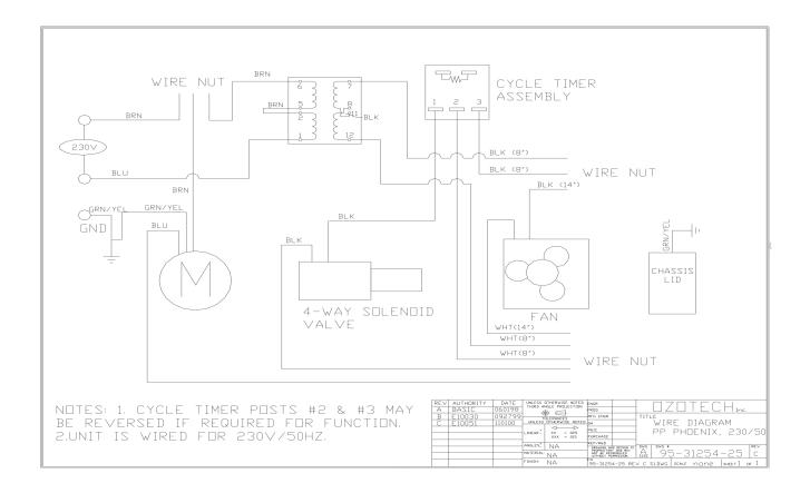
FIGURE 4 - Wiring Diagram, Power Prep Phoenix, 230Vac/50Hz
