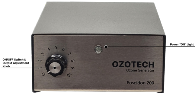
Figure 3. Poseidon 200 Ozone Generator (Front View)
