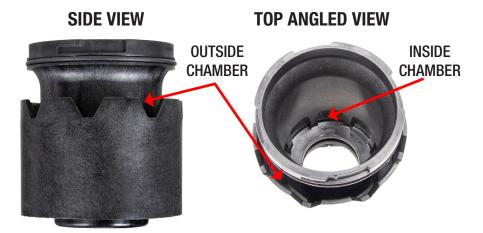
Air Blocker traps water in its chambers, blocking the head of air in the tank from entering the control valve, reducing iron oxidation in the valve.
